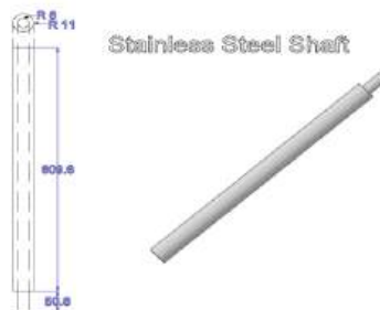
Rajah 3.5: Aci ( Stainless steel shaft )
