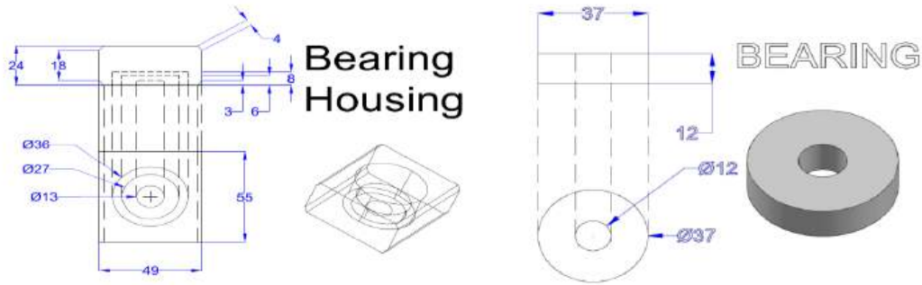
Rajah 3.3: Rumah gelas bebola ( Bearing housing )
