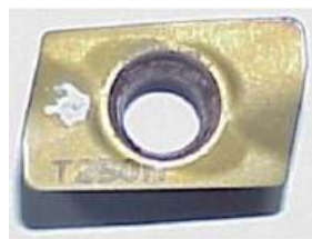
Figure 5: CVD coated carbide tool
